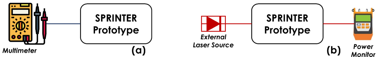
Figure 1: Indicative schematic representation of the “static” measurements’ experimental setup. (a) Electrical (b) Optical
