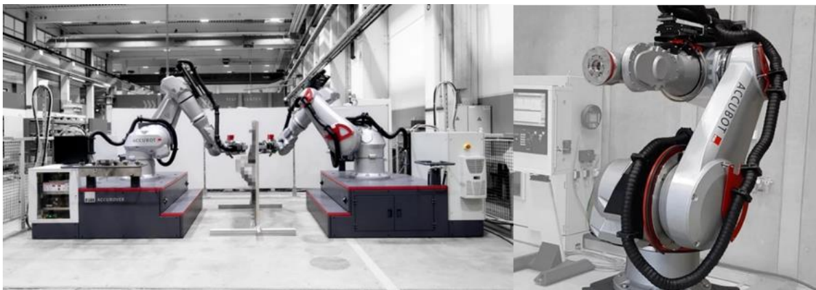
Figure 18: Accubot in the Fill NC Robot Lab and Dual Robot NDT cell.
